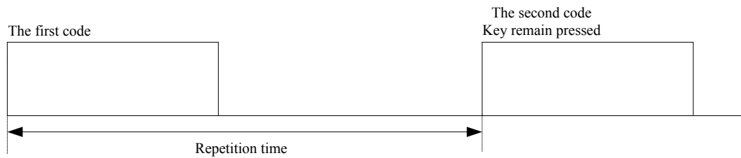
Figure 10-9 RC5 Protocol of Repetition time
