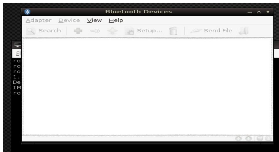
5. Upload the bluetooth firmware.(Cubieez system can directly execute the script open-bluetooth.sh to do this)
