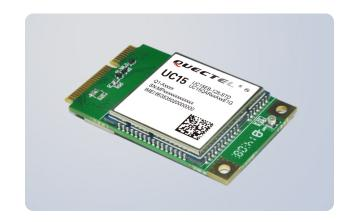
UC15 Mini PCIe is a UMTS/HSDPA module featuring a maximum data rate of 3.6Mbps downlink and 384Kbps uplink. It is designed to provide customers with global network coverage on the connectivity of HSDPA/WCDMA, and it is also fully backward compatible with existing EDGE and GSM/GPRS networks through multi-band combination of dual-band WCDMA and dual-band GSM.
